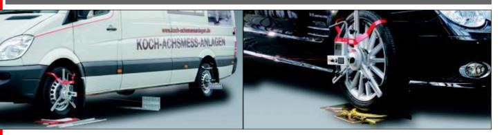
**AL-30**, **for measuring trucks and trailers:** trucks and trailers are measured and adjusted from the axles to the measurement traverse AL-30 on the reference point – king pin or drawbar eye. This is done with HD-30 laser measurement heads.
